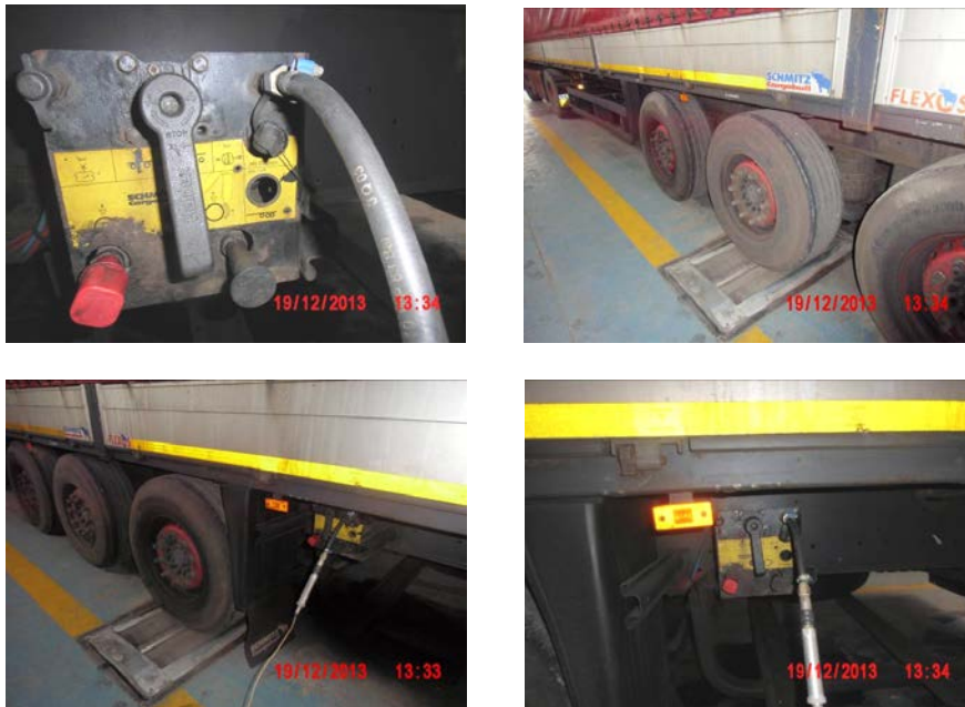
Fig. 5. Testing the brake system of the SCHMITZ SPR24 2002 trailer
